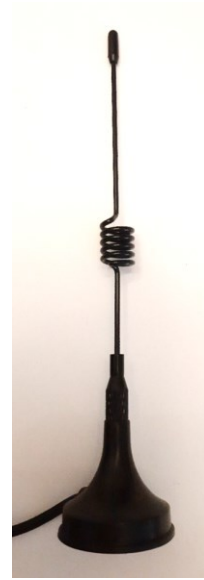
Figure 3. 433 MHz antenna with a gain of 5dBi.
