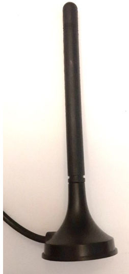
Figure 2. 433 MHz antenna with a gain of 3dBi.
